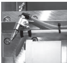
A smart and environmental friendly lubrication system extends tool life without excessive spilling keeping the machined product clean
